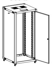
ISOMETRIC REAR VIEW WITH CASTER SET WITH HINGED REAR DOOR
