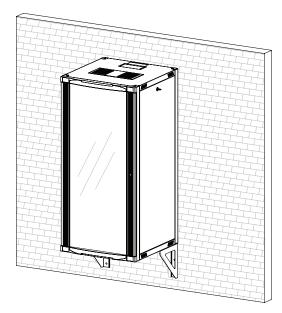
ISOMETRIC VIEW WITH WALL SUPPORT BRACKETS
